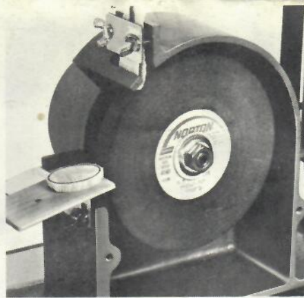
Grinding to mark with bezel angle table furnished with CAB-MATE. Makes correct bezel angle automatically.
